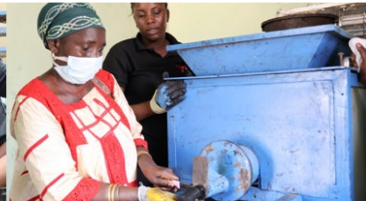
Maguette cuts the moulded biochar pieces as they come off the machine.
